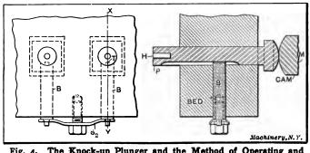
Fig. 4. The Knock-up Plunger and the Method of Operating and Retaining it
